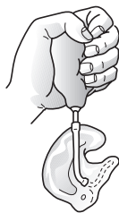
Use air bulb to remove residual water.
